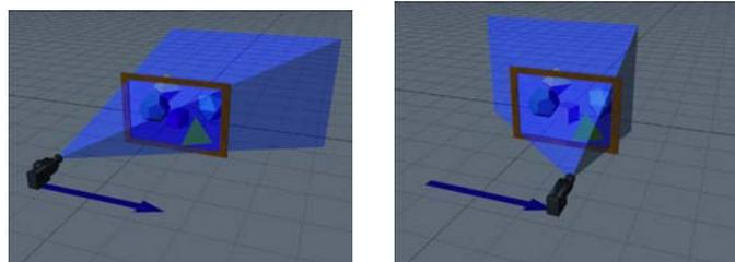
Fig. 1 & 2: Virtual camera setup of a computer generated holographic panoramagram.
